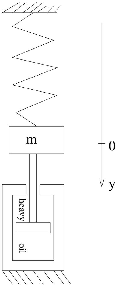
A mass with a spring and a shock absorber
