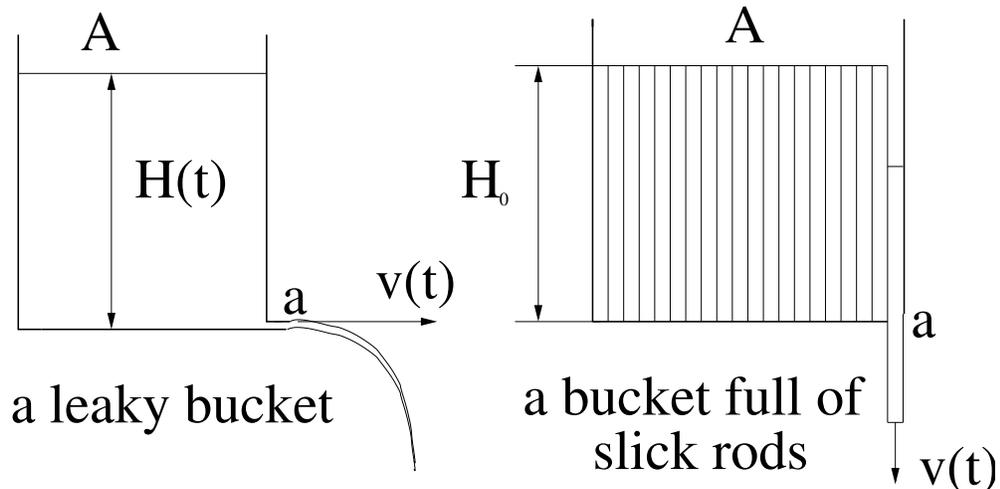
Let  $A$  be the area of the horizontal cross-section of the bucket,  $a$  be the area of the hole and  $H_0$  be the original water level in the bucket. Assume that the hole in the bucket was opened up at time 0, so  $H(0) = H_0$  where  $H(t)$  is the water level at time  $t$ .
