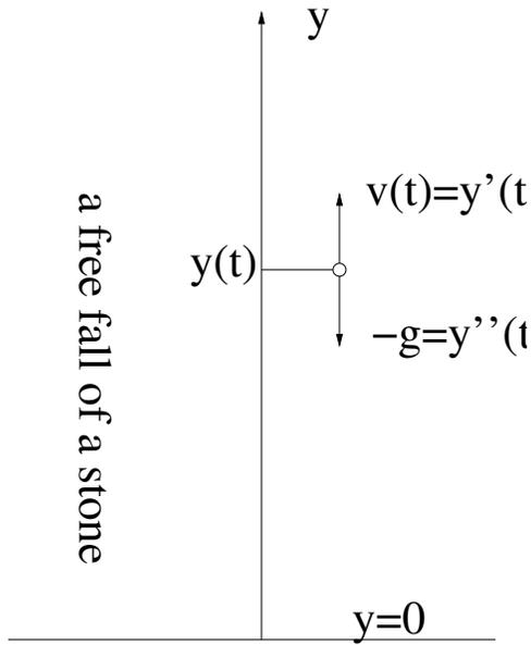
It follows from Newton's Second law:  $F = ma$ , where  $m$  is the mass of the stone,  $a = y''$  is its acceleration and  $F = -gm$  is the force of gravity. We also have two additional conditions:
